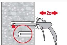
Blow again with compressed air 4 times until return air stream is free of noticeable dust.
