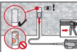
Overhead installation and/or installation with embedment depth  $h_{ef} > 250\text{mm}$ .
