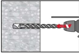
Drill with hammer drill a hole into the base material to the size and embedment depth required by the selected anchor (Table B2).
