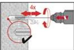
Check brush diameter (Table B2) and attach the brush to a drilling machine or a battery screwdriver. Brush the hole with an appropriate sized HIT-RB wire brush (Table B4) a minimum of four times.
