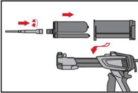
Tightly attach new Hilti mixing nozzle HIT PM to foil pack manifold (snug fit). Do not modify the mixing nozzle.
