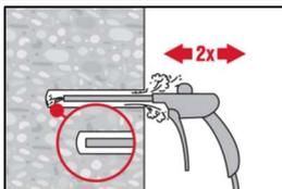
Blow 4 times from the back of the hole (if needed with nozzle extension) over the hole length with oil-free compressed air (min. 6 bar at 6 m<sup>3</sup>/h) until return air stream is free of noticeable dust.
