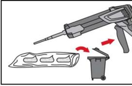
Prior to dispensing into the drill hole, squeeze out separately a minimum of three full strokes and discard non-uniformly mixed adhesive components until the mortar shows a consistent grey colour. For foil tube cartridges it must be discarded a minimum of six full strokes.
