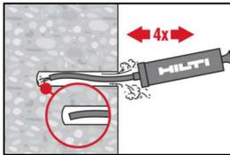
The Hilti hand pump may be used for blowing out drill holes up to diameters  $d_0 \leq 20$  mm and embedment depths up to  $h_{ef} \leq 10 \cdot d$ .
