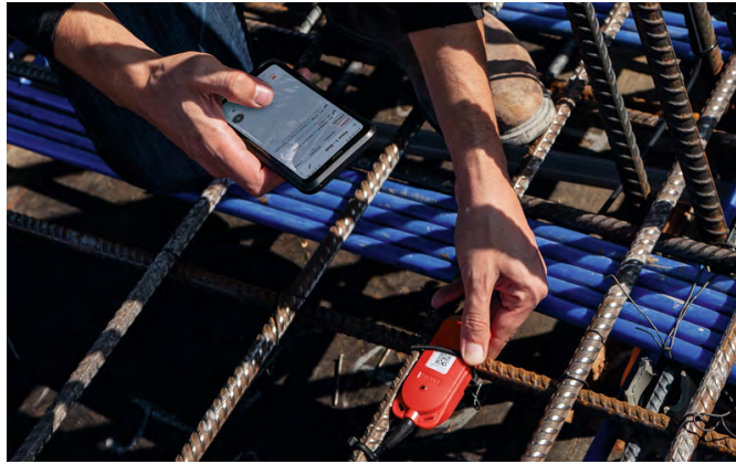
Fig.9.20: Hilti concrete sensor (wireless) that transmits real-time data on concrete temperature, strength and relative humidity onto the concrete sensors mobile application
