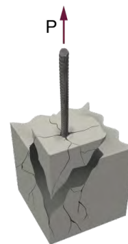
Fig. 2.11: Concrete cone breakout failure
