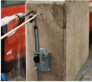
Fig. 9.7: Example of drilling aid
