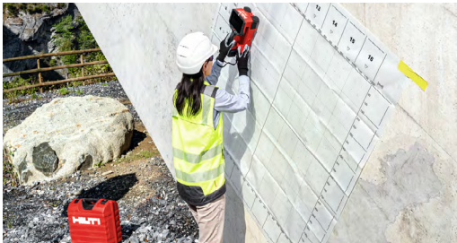
a) Scanning for ferrous objects
