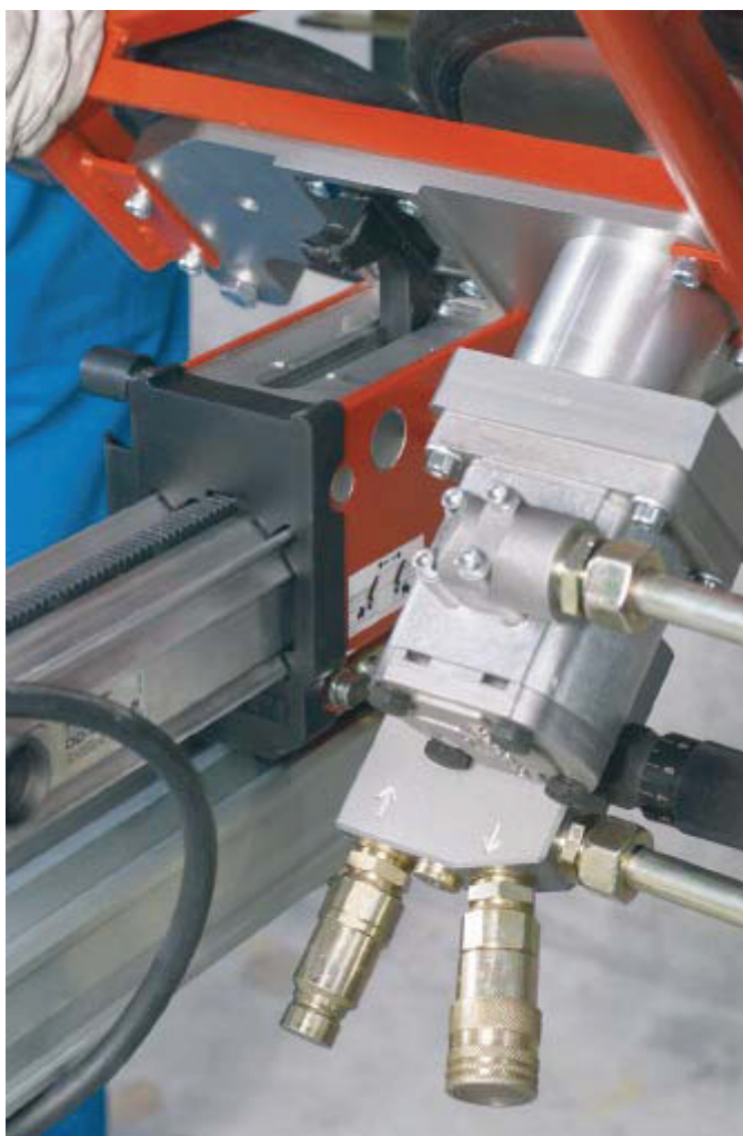
Spanhaak in opnamesleuf inbrengen
